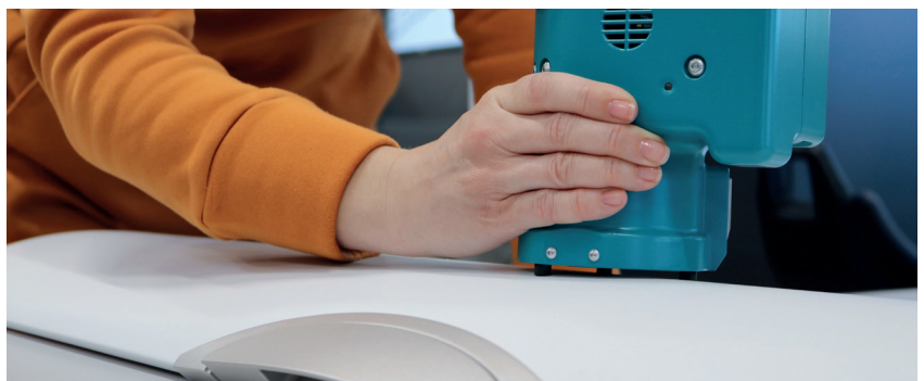
T-SCAN testing an airplane overhead compartment
