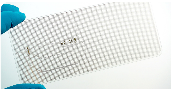
Printed semi-transparent conductors for smart window applications
