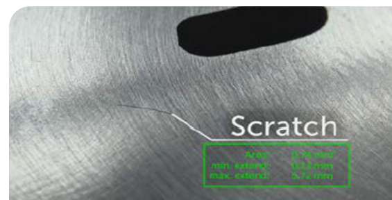
Labeling of defect classification and defect parameters
