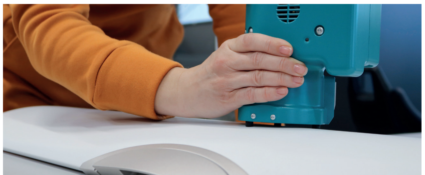
T-SCAN testing an airplane overhead compartment
