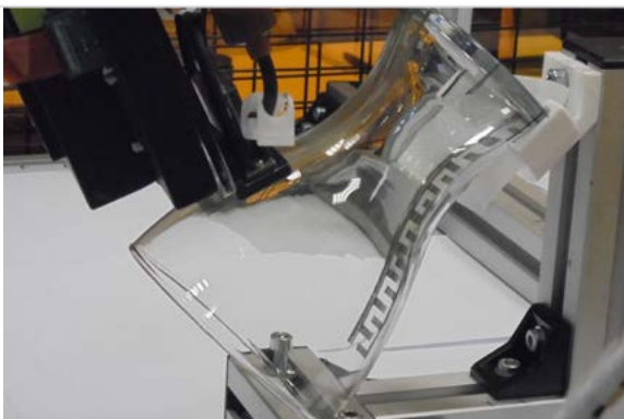
Printing conductive inks on curved glass
