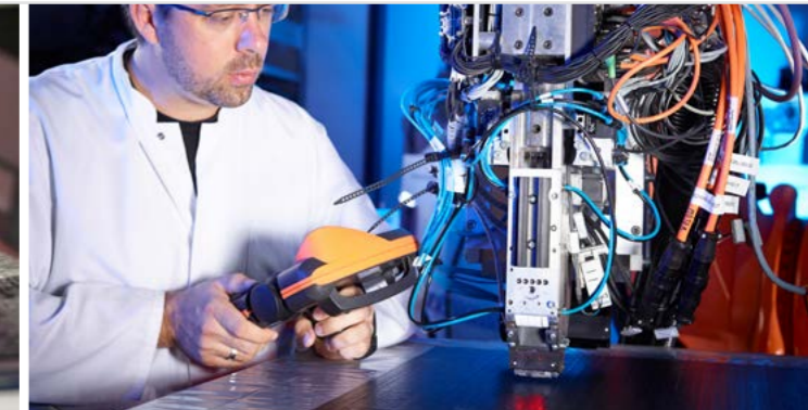
The L-Scan provides depth images for inspecting the edges of the individual carbon fibre tows.
