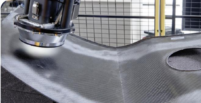
Inspection of carbon composite components and materials
