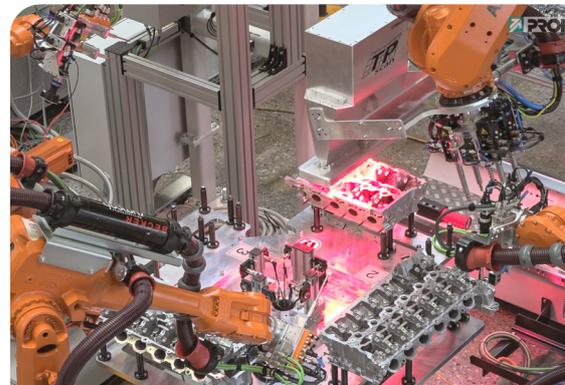
Complete solution for the inspection of engine blocks
