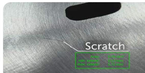
Labeling of defect classification and defect parameters
