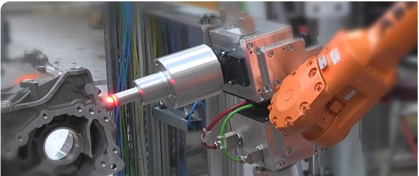
D20-F rotating sensor during hole inspection
