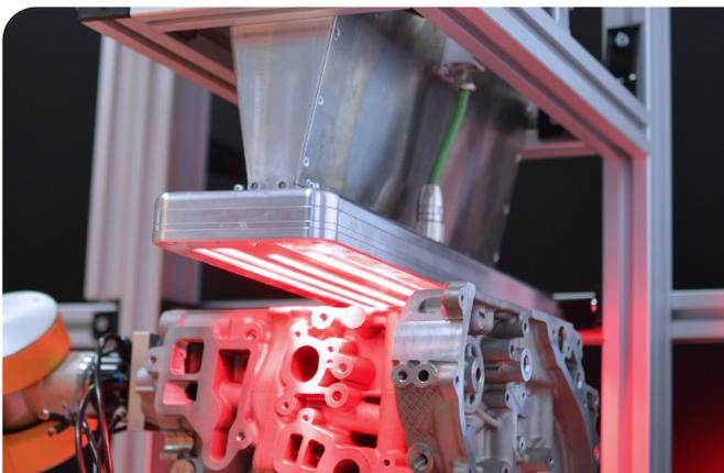
Engine block inspection with TPScan Sensor 400
