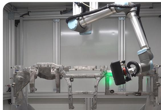
Complete solution for the inspection of aluminum structural components
