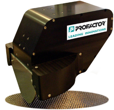
FILA INSPECT inspecting a carbon fibre mat
